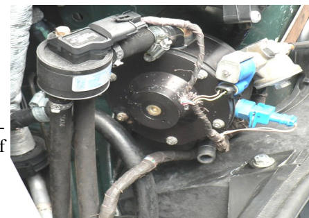
Prins LPG system. The reducer is the large black circular unit that has liquid LPG fed one side of a rubber diaphragm and engine coolant the other. As coolant heats up, the liquid LPG evaporates into a gas suitable for cylinder combustion. The heat up is monitored turning off petrol when gas pressure's sufficient
