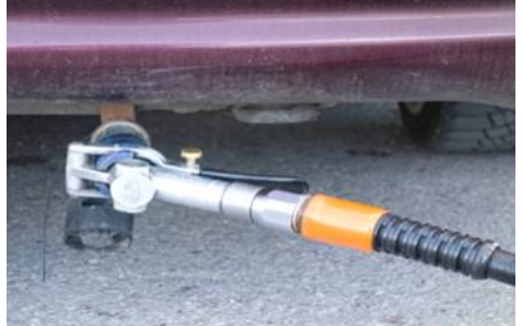
A UK-style lever Bio-LPG nozzle connected to a converted vehicle's fuel tank. Another nozzle style found in UK uses a rotating ring to lock
