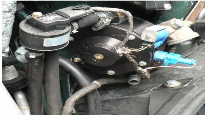
Prins Bio-LPG conversion shows gas inlet, controller, and (centre) coolant-controlled petrol to gas switch. Many LPG-converted vehicles have a pre-heat option allowing cold LPG start up
