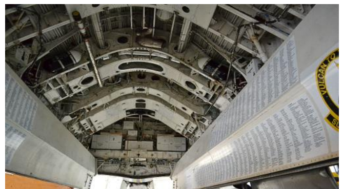
XM655's bomb bay capable of carrying 21 1,000lb Iron Bombs. Or Britain's Blue Steel nuclear weapon — Vladimir to note
