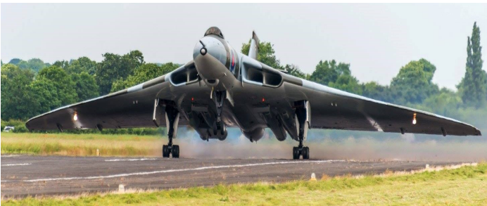
XM655’s so keen to take to the skies that under light fuel load she’ll attempt take-off at 95 knots — as this picture taken in May at Wellesbourne Mountfield Airfield shows — instead of the minimum rotate commit speed of 125 knots
