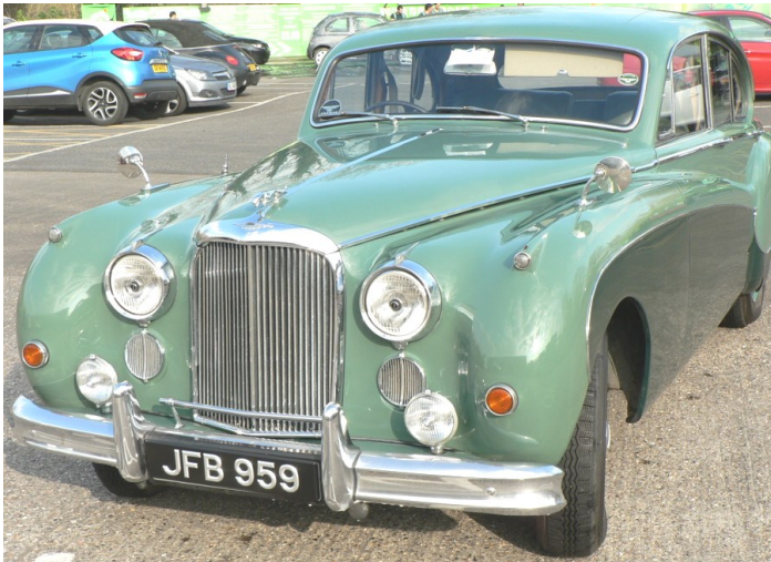
1959-registered Jaguar Mk IX. Star of the Alfred Hitchcock film Vertigo. 3781cc twin overhead cam XK engine producing 220BHP
